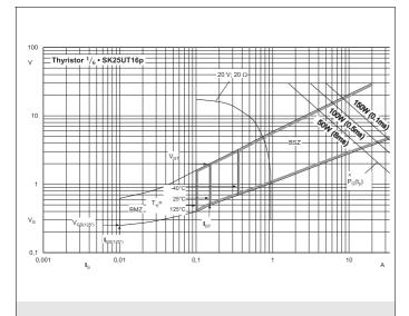
Fig. 5: Gate trigger characteristic
