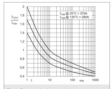
Fig. 4 : Surge overload current vs. time
