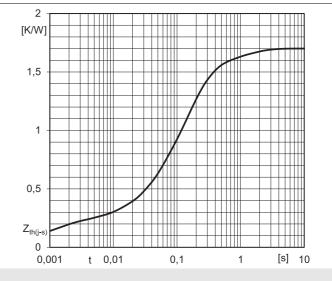
Fig. 2: Transient thermal impedance vs. time
