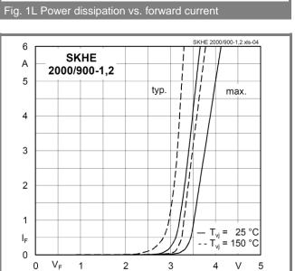
Fig. 4 Forward characteristics
