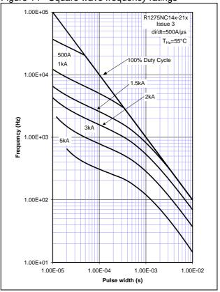
Figure 15 - Square wave frequency ratings
