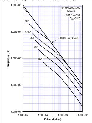
Figure 14 - Square wave frequency ratings
