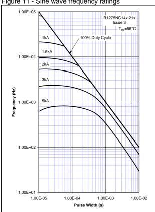
Figure 12 - Sine wave frequency ratings
