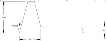
The magnitude of  $I_{GM}$  should be between five and ten times  $I_{GT}$ , which is shown on page 2. Its duration  $(t_{p1})$  should be 20µs or sufficient to allow the anode current to reach ten times  $I_L$ , whichever is greater. Otherwise, an increase in pulse current could be needed to supply the necessary charge to trigger. The 'back-porch' current  $I_G$  should remain flowing for the same duration as the anode current and have a magnitude in the order of 1.5 times  $I_{GT}$ .
