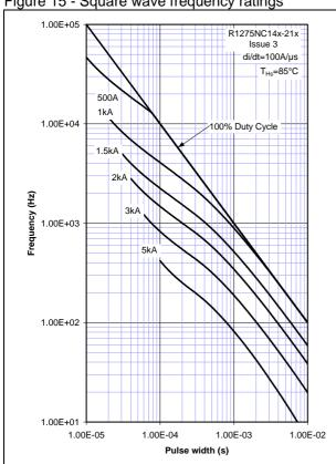
Figure 16 - Square wave frequency ratings
